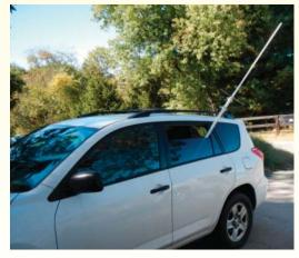
for more than a few miles. It is just about perfect for use while sitting in the portable chair. I have since fashioned a clip to hold the speaker mic on the mast next to the HT. I found that the antenna was unstable with a mast more than 10 feet in length. Works great sitting in the place of an umbrella in a patio table.
