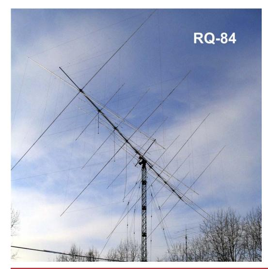
To the left is a picture of R-Quad's Model RQ-84 cubical quad antenna for the HF ham bands.
