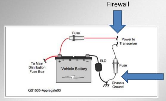
Older vehicles (without ELD): negative fuse lead directly to battery negative terminal.
