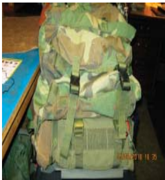
A backpack radio on a surplus pack frame. A small shelf holds the battery and allows the pack to stand upright.
