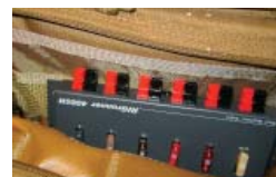
The front pocket holds a Rig Runner for fuses and power distribution.
