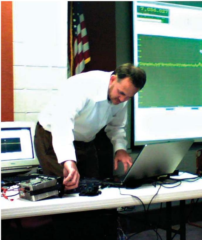
computer via a USB cable. See image to the left. The laptop processed the IQ audio signals using MØKGK's software for a Software Defined Radio. Go to MØKGK's website [<http://www.m0kgk.co.uk/sdr/>] for more information and a free download of that software.
