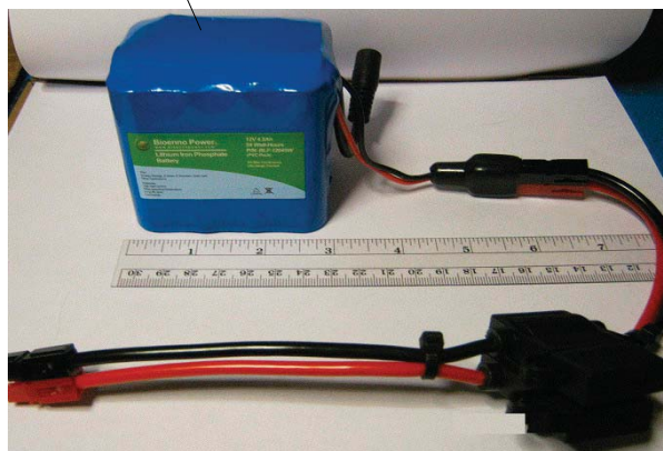
My 4.5 Ah mini LiFePO4 and fused cable. (The battery came with Power Pole output connector.)
