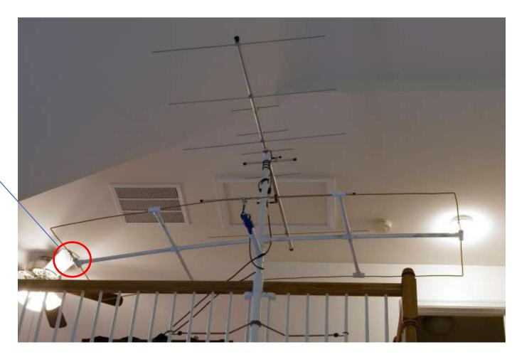
You may also tune the antenna by expanding the width a bit. That requires re-bending the wire.
