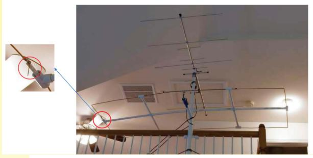
You may also tune the antenna by expanding the width a bit. That requires re-bending the wire.
