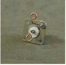
Just about ready. You must make the last reflector bend after inserting the wire in the frame.
