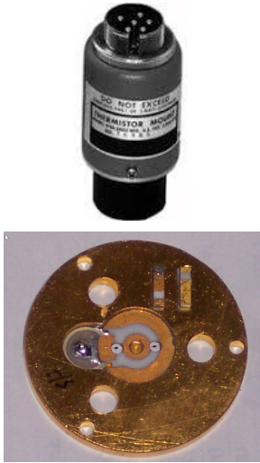
Figure 2-2. Simplified diagram of the HP 478A dual-element temperature compensating, coaxial thermistor mount.
